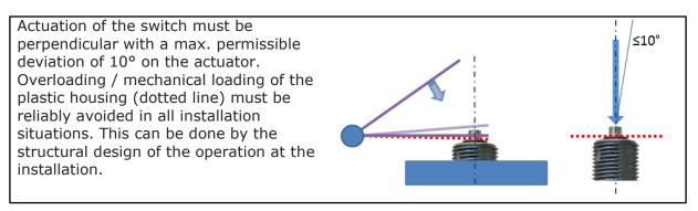
The Microswitch M12 must be installed protected from the risk of mechanical danger, under consideration of the above mentioned operating conditions. This can be done constructively e.g. by installation in a protecting enclosure, or the use of a suitable actuator, when installed in a housing wall by protected installation, a protective collar or by a metal sleeve with the minimum wall thickness of 2mm is needed.
